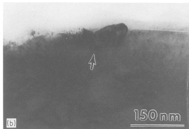
Figure 8 TEM images of samples deposited and annealed for 2 hours at 525 °C. The arrow in (b) indicates the Ti_3Al phase. The Ti_3Al is not continuous in this region.
